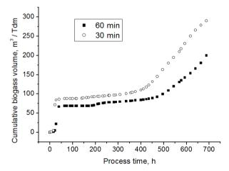
Fig. 4. Time-course of batch methane-fermentation of straw samples being subjected to preliminary steam-explosion process in temperature of 180°C
