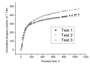
Fig. 2. Time-course of batch methane-fermentation of poultry manure premixed with sawdust
