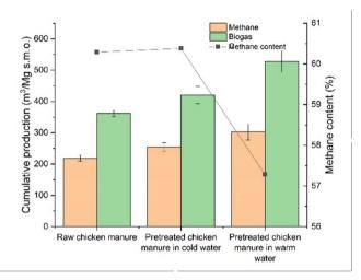
Fig. 3. Cumulative biogas and methane production for raw and pretreated chicken manure
