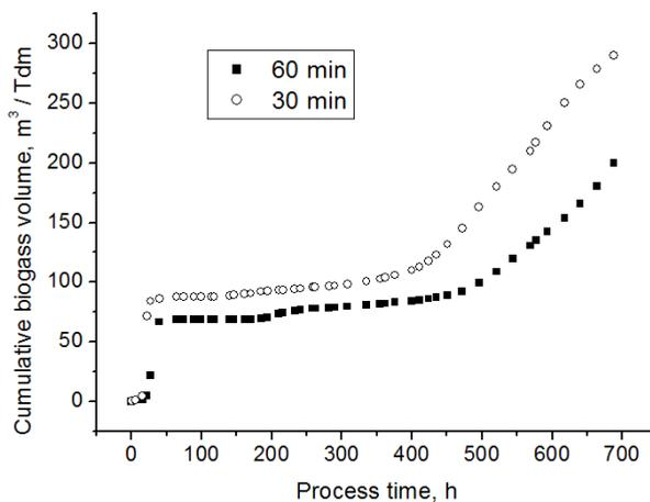
Fig. 4. Time-course of batch methane-fermentation of straw samples being subjected to preliminary steam-explosion process in temperature of 180°C
