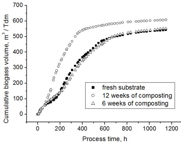
Fig. 5. Time-course of batch methane-fermentation of poultry manure premixed with the straw (room with floor heating system) — “fresh” substrate, after 6 and after 12 weeks of composting (aeration)
