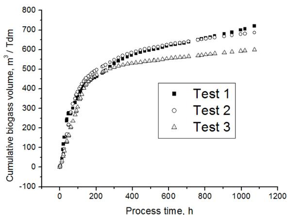
Fig. 3. Time-course of batch methane-fermentation of poultry manure premixed with the straw
