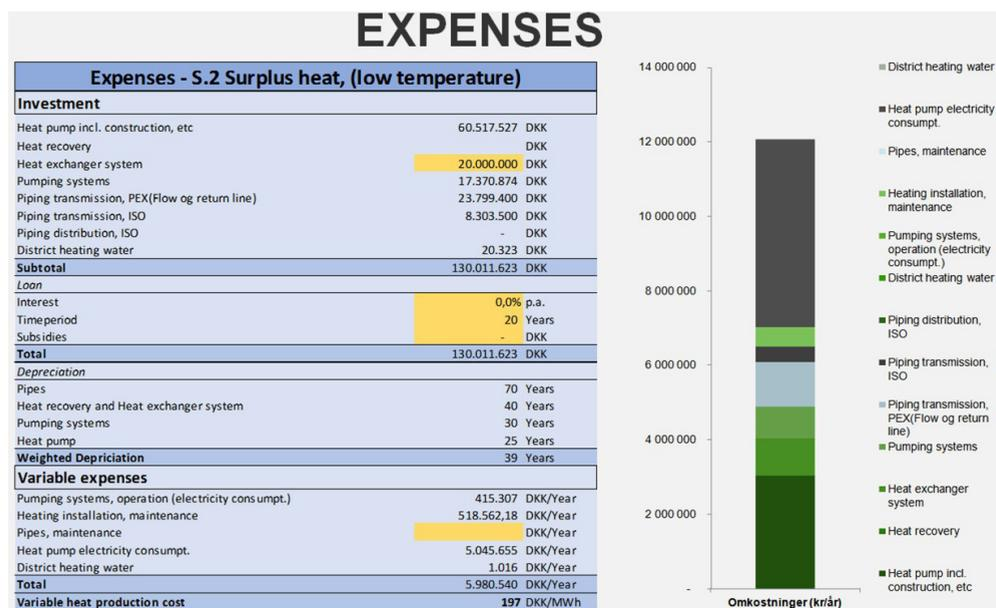
Fig. 7. Economy of long distance, low temperature LTDH (~300 K) — 20 km long distance (19 km uninsulated transmission using PEX pipes to central heat pump, later insulated transmission (1 km) using ISO pipe at temperature 75°C)
