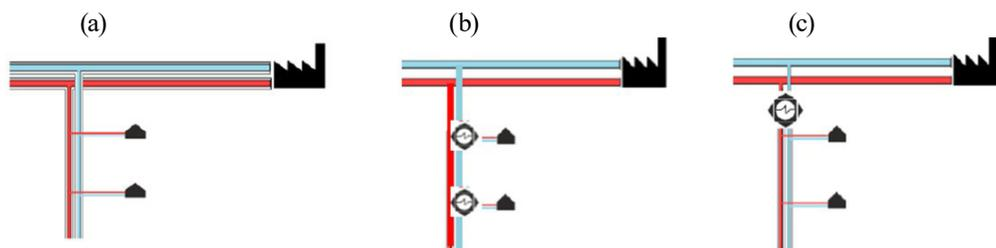
Fig. 6. The considered options: (a) insulated transmission, (b) uninsulated transmission line to the individual heat pumps, (c) uninsulated transmission line to the village and general heat pump (after D. Marhauer-Nimb, Energy Efficient Cities Conference, 2018, Gdynia)
